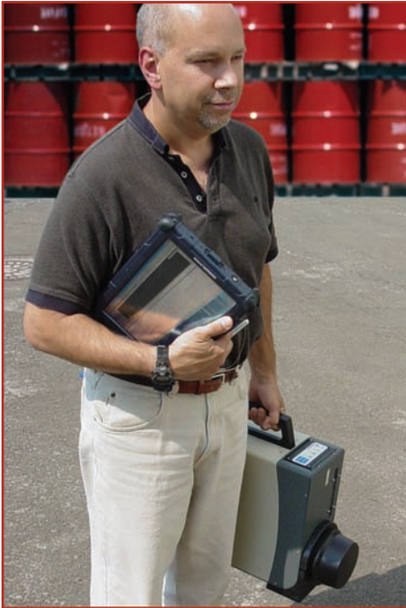
The Falcon is a radionuclide identifier (based on a high-purity germanium (HPGe) detector). It quickly answers: "Is there a radiation source present?"; "Where is it?"; and, importantly, "What isotopes are emitting the radiation?"
