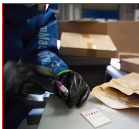
An actual evaluation of a suspicious white powder from a mailing envelope using ADVNT Biotechnologies' ProStrips 5 biothreat hand-held assay.
