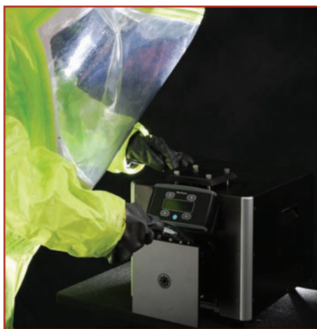
The BioFlash™ is a highly portable, high-performance, easy-to-use integrated aerosol sampler and identifier that is used specifically for biodefense applications.
