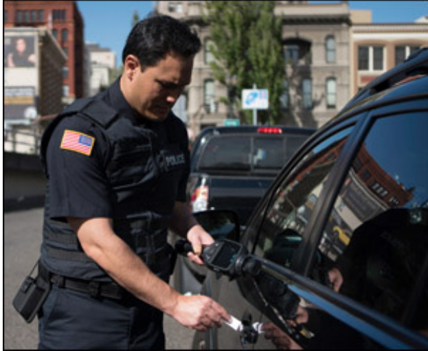
Handheld explosives trace detector. Source: FLIR Systems Inc. (2015).
